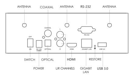
Antenna Installation Instruction: Please install the three antennas from the accessories onto the antenna interfaces shown in the image above.
