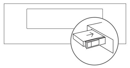
**Note:** Do not load or replace the hard disk while the device is powered on to avoid damage to the device or hard disk data. Brand new hard disks need to be formatted before loading. This device supports the following hard drive formats: EXT3, EXT4, NTFS, FAT32, EXFAT
