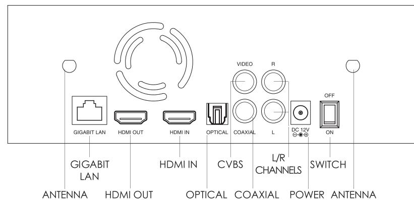
Instruction to installation of the antenna: Please insert the two antennas in the parcel into the antenna ports in the above diagram.
