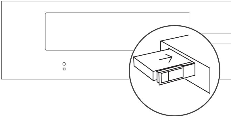
Note: Do not load or change the hard disk while the power is on to avoid that the device or the data of hard disk be damaged. If it is a brand-new hard disk, please format it before loading it to the device. This device support following formats of hard disk: EXT3, EXT4, NTFS, FAT32, EXFAT.
